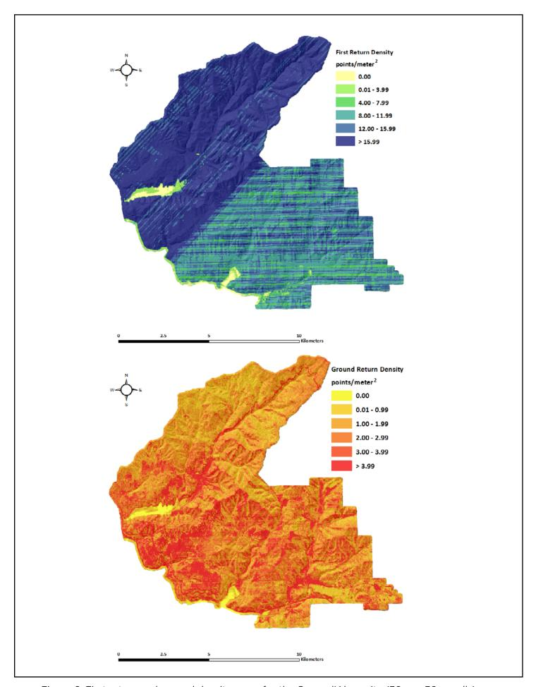
Figure 6: First return and ground density maps for the Coeur d'Alene site (30 m x 30 m cells)
