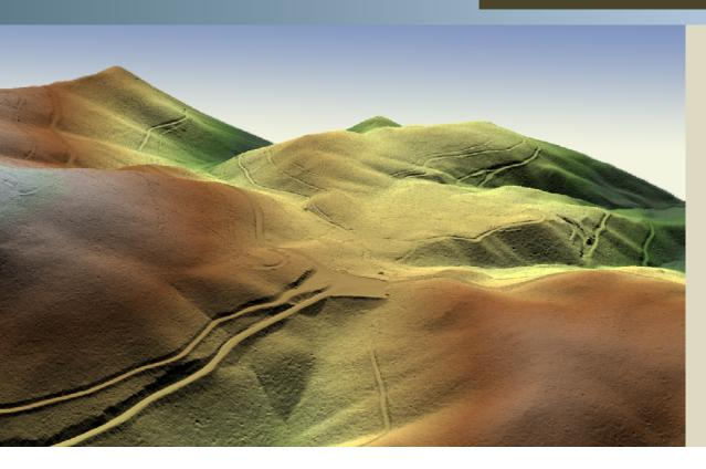
View looking southeast at Fernan Saddle. The image was created from the gridded LiDAR surface colored by elevation.
