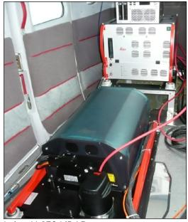
Leica ALS70 LiDAR sensor
