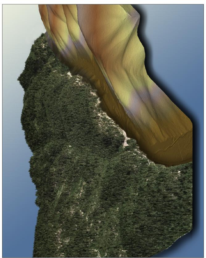
Forest Service Road 268. The image was created from the gridded LiDAR surface colored by elevation with a portion of the bare Earth image overlaid with the 3-D LiDAR point cloud and National Agriculture Imagery Program (NAIP) imagery. Figure 9: View looking northeast at the point where E. Fernan Lake Road forks into E. Forest Service Road 1562A and N.
