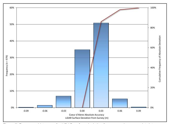
Figure 11: Frequency histogram for LiDAR surface deviation from ground survey point data.
