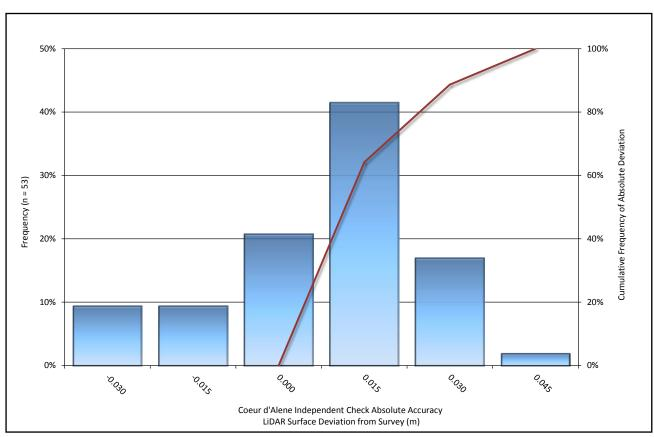
Figure 7: Frequency histogram for LiDAR surface deviation from reserved ground survey control point data.
