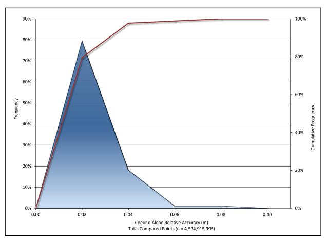
Figure 8: Frequency plot for relative vertical accuracy between Coeur d'Alene flightlines
