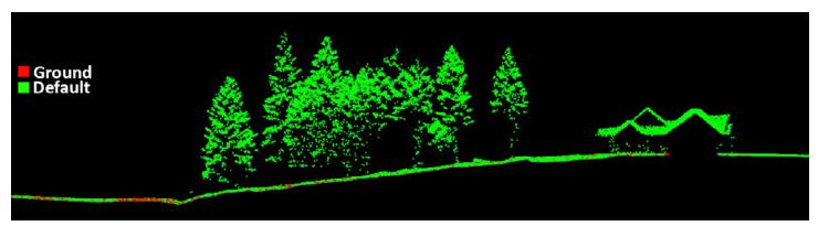
View of a house next to a grove of conifer trees located in Bennett Bay. The image was created from a 3 meter cross section of the 3-D LiDAR point cloud and colored by point classification.
