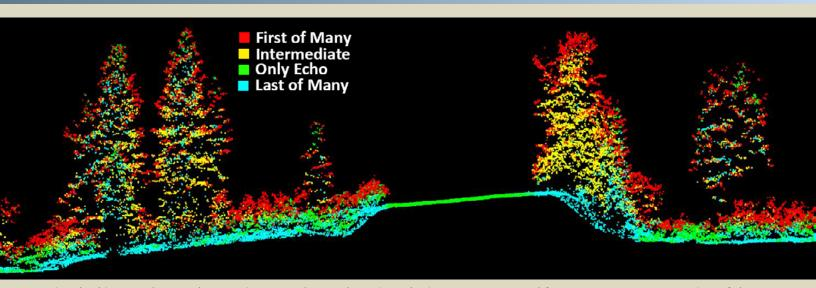
View looking northwest along E. Coeur D'Alene Lake Drive. The image was created from a 3 meter cross section of the 3-D LiDAR point cloud and colored by echo.
