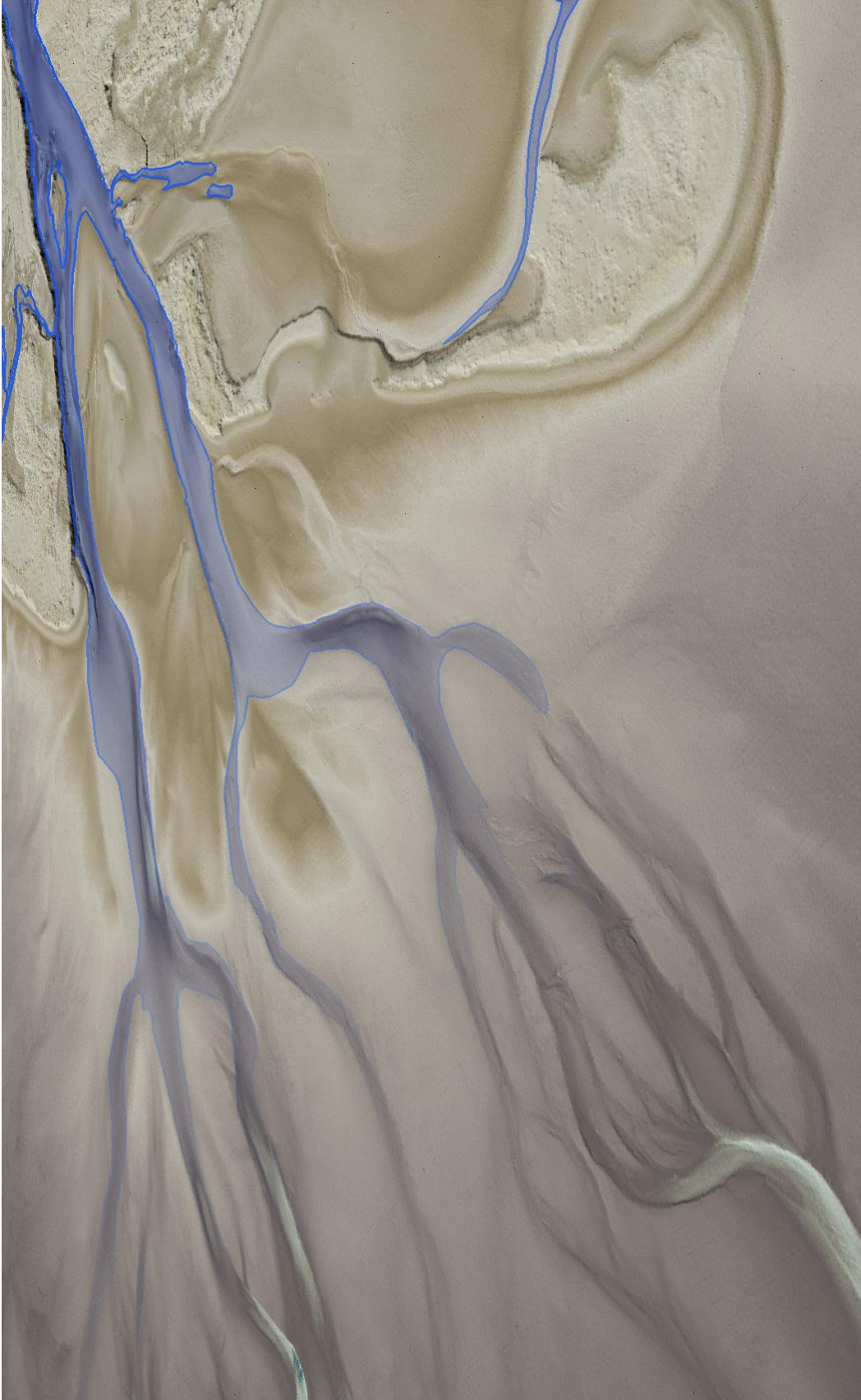
Figure 21: View of the mouth of the Dungeness River. The image is created from the gridded, bare earth and bathymetric bottom LiDAR returns colored by elevation, overlaid with the water's edge breaklines
