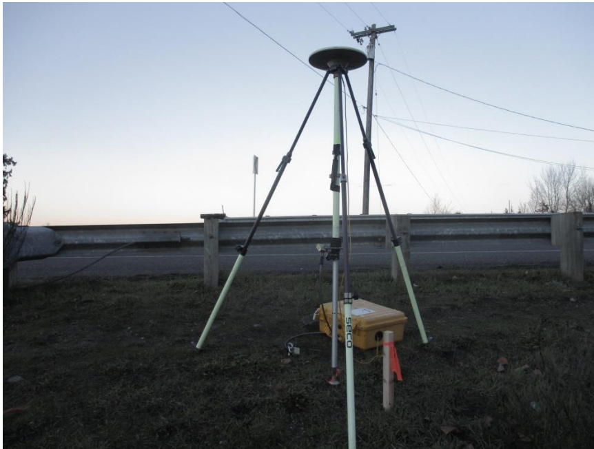
Top image: QSI ground survey equipment set up over monument DUNGENESS_01.
