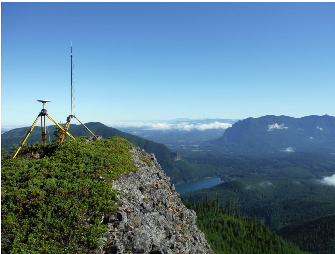
This photo taken by QSI ground acquisition staff shows a view of the Trimble R7 GNSS system set up on a hilltop in the Cedar Watershed project area.
