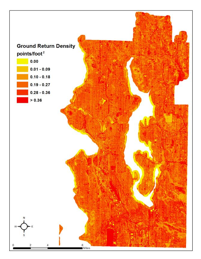
Figure 6: Ground density map for the King County Delivery 1 site (100 m x 100 ft cells)
