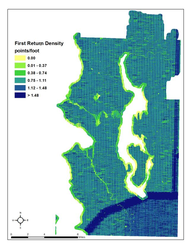
Figure 5: First return classified point density map for the King County Delivery 1 site (100 ft x 100 ft cells)
