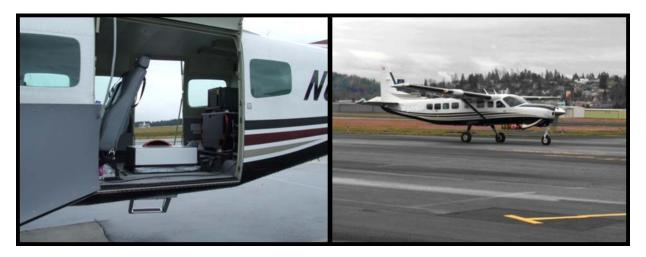
The Cessna Caravan is a stable platform, ideal for flying slow and low for high density projects. The Leica ALS50 sensor head installed in the Caravan is shown on the left.
