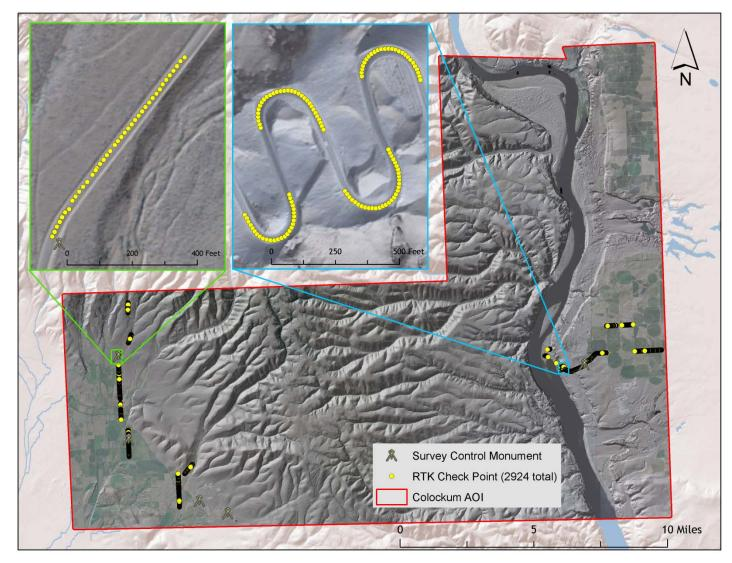
Figure 2. RTK check point and control monument locations used in the Colockum AOI
