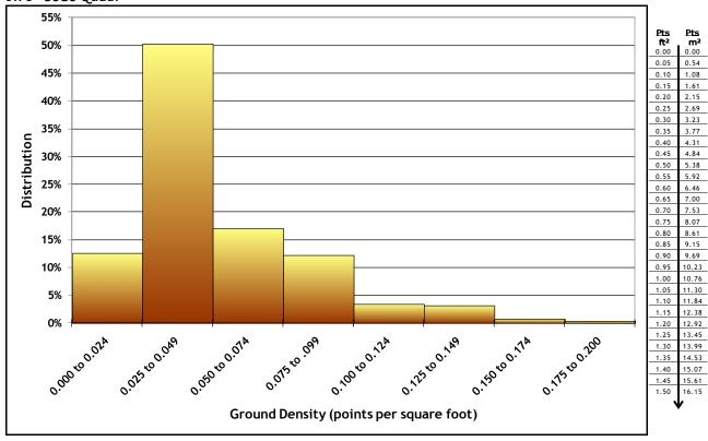
**Figure 4.10**. Image shows ground-classified laser point density for in the Lewis County study area, per 0.75' USGS Quad.
