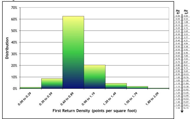
**Figure 4.8.** Image shows first return laser point density for in the Lewis County study area, per 0.75' USGS Quad.
