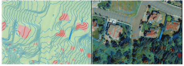
The CAD files (\*.DWG) are coded to display high and low confidence contours as green and red, respectively (Figure 3.2). The elevation label units are feet.
