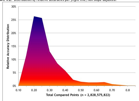
Figure 4.2. Distribution of relative accuracies per flight line, non slope-adjusted.
