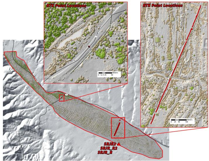
Figure 3. Base station locations and 544 RTK point locations in the Sumpter AOI. RTK detail views shown over 1-meter Above Ground ESRI Grid.
