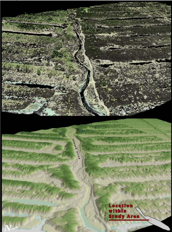
**Figure 14.** 3-d oblique view of LiDAR-derived surfaces in processing bins 27-29, showing a short section of the Powder River, at the southeastern edge of the Sumpter AOI. (Top image derived from all points, bottom image derived from ground-classified points).
