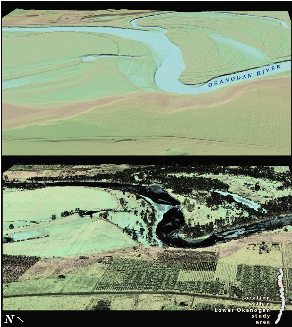
Figure 53. 3-d oblique view of LiDAR-derived surfaces in the southern portion of quad 48119-H4 of the Okanogan River in the Lower Okanogan, Washington study area. (Top image derived from ground-classified points, bottom image derived from all points).
