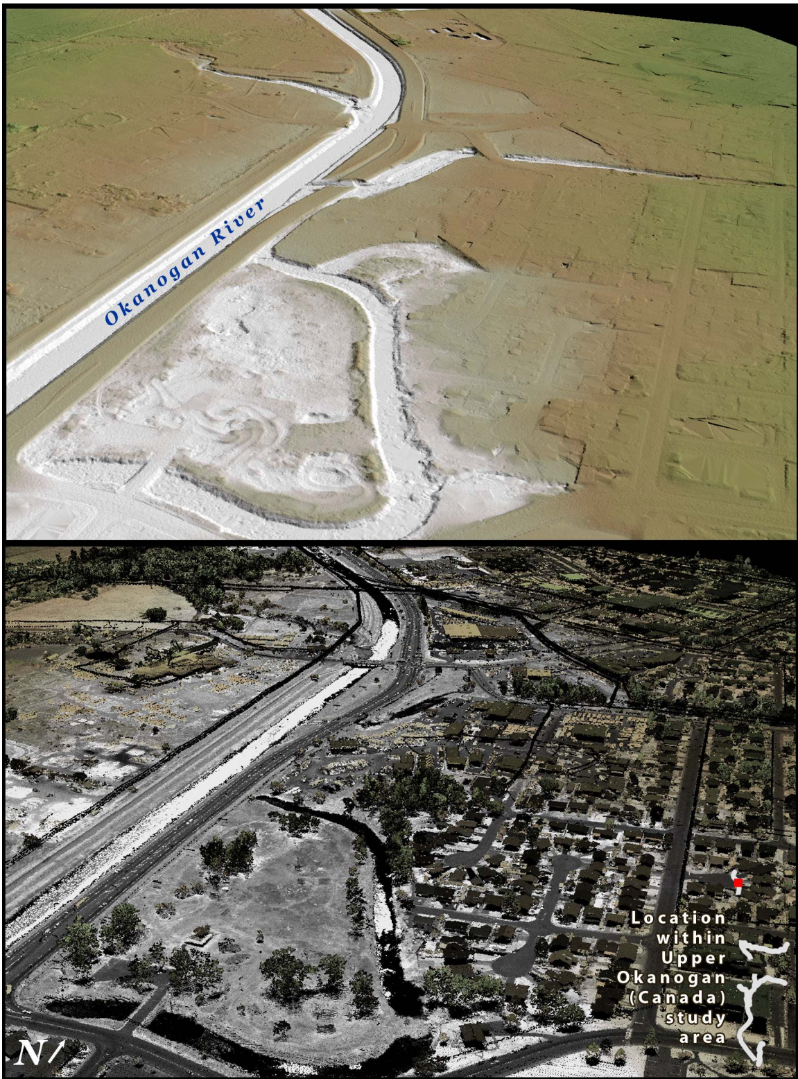
Figure 45. 3-d oblique view of LiDAR-derived surfaces in the central portion of quad 49119-D5 along the Okanogan River in the Upper Okanogan, Canada, study area. (Top image derived from ground-classified points, bottom image derived from all points).
