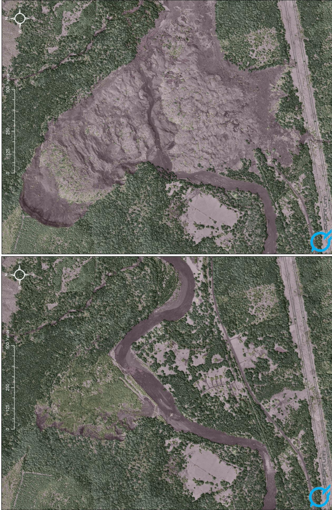
Figure 11: A view showing the shaded terrain of the Oso Landslide site before and after the event. The left image shows the site using data collected by QSI in July of 2013, and the right image shows the same view in March of 2014. The bare earth models are overlain with the above-ground LIDAR point cloud.
