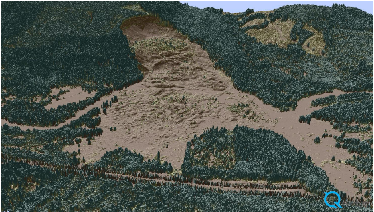
Figure 13: A 3D view showing the shaded terrain of the Oso Landslide site before and after the event. The top image shows the site using data collected by QSI in July of 2013, and the bottom image shows the same view in March of 2014. The bare earth models are overlain with the above-ground LiDAR point cloud.
