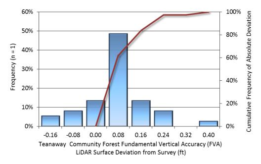
Figure 7: Frequency histogram for LiDAR surface deviation from ground survey point values
