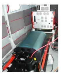
Leica ALS70 LiDAR sensor
