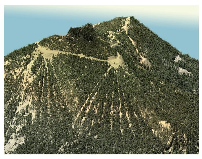
Figure 10: View looking West at two old cable logging corridors. The image was created from the gridded LiDAR surface colored by elevation and overlaid with the 3D LiDAR point cloud.
