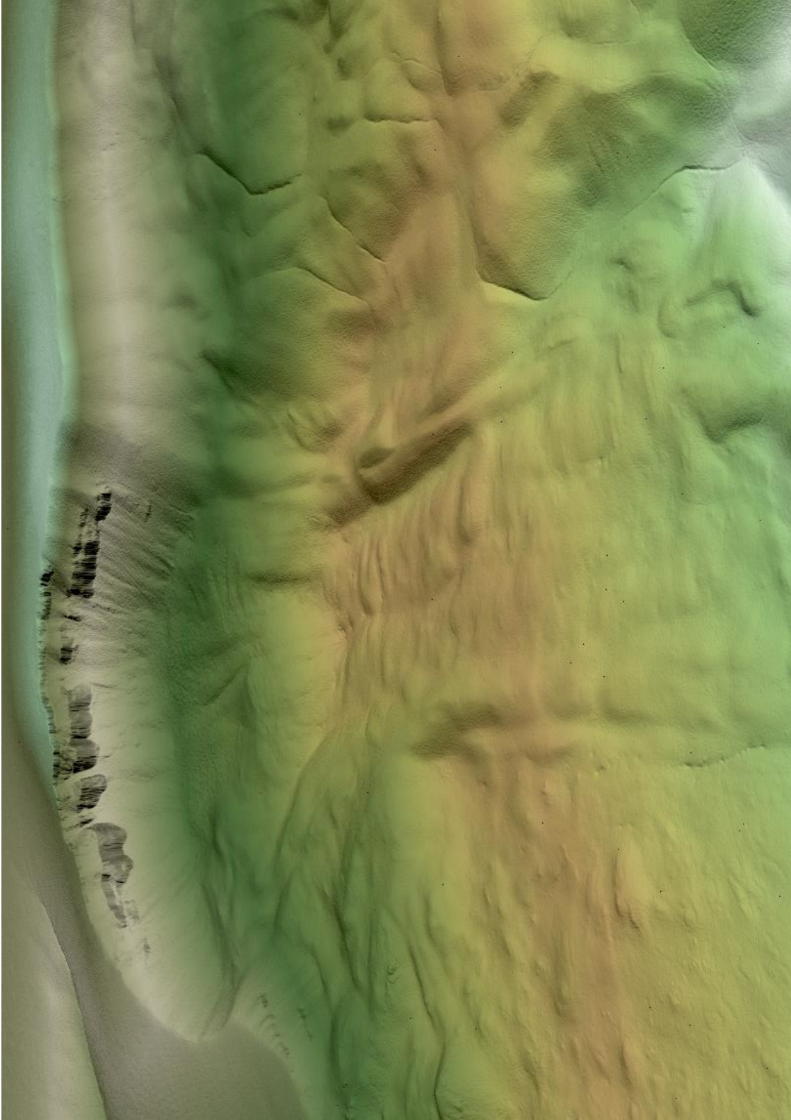
Figure 9: A view looking southeast at a scarp in the Saddle Mountains. Image created from the gridded ground-classified LiDAR points colored by elevation.
