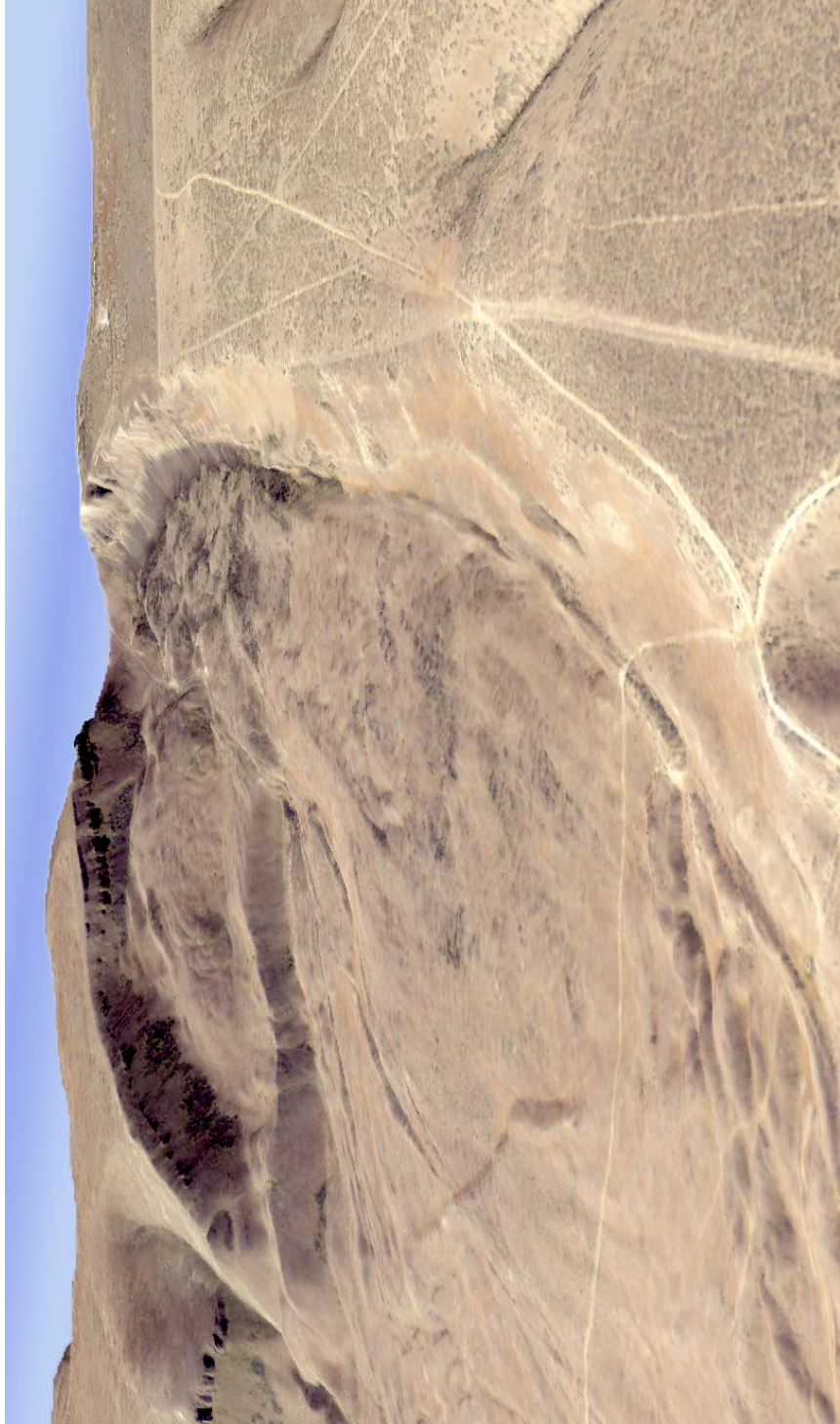
Figure 8: A view looking south at a historic landslide in the Saddle Mountain study area. The image was created from the LiDAR point cloud with RGB values assigned from 2009 NAIP imagery.
