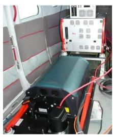
Leica ALS70 LiDAR sensor
