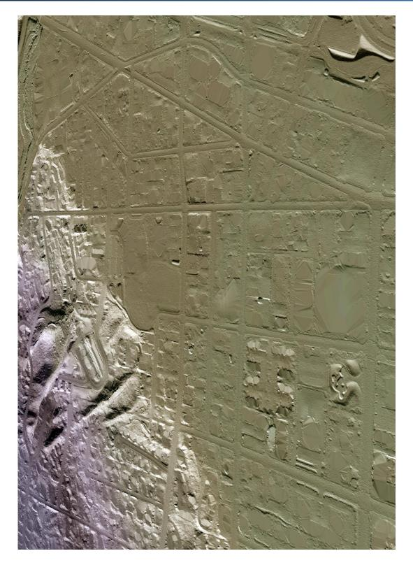
Figure 9: View looking west over downtown Redmond. The image was created from the bare earth LiDAR model colored by elevation.
