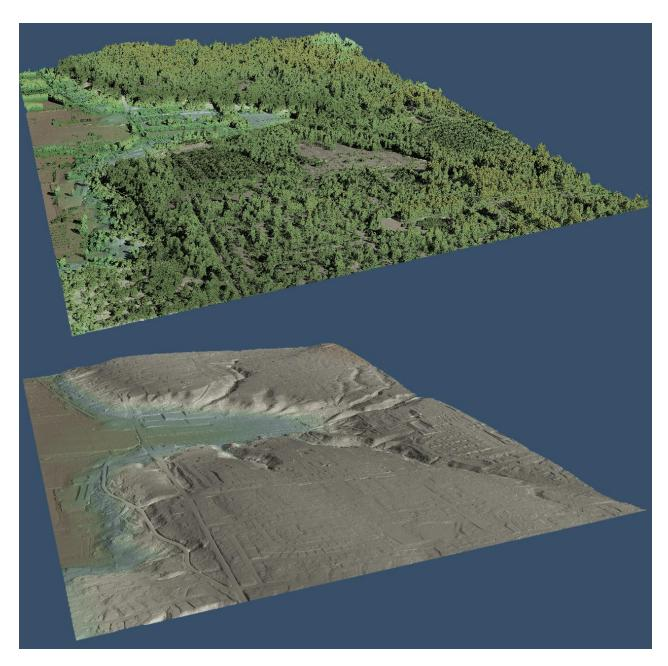
Figure 10: The bottom image is a bare earth model colored by elevation looking northeast over north Redmond. The top image is the same view, but overlain by the above-ground LiDAR point cloud.
