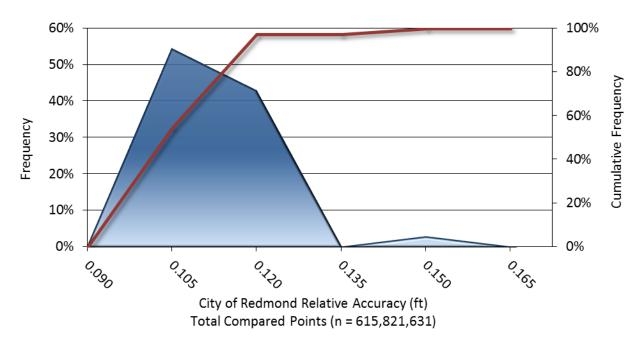
Figure 8: Frequency plot for relative vertical accuracy between flight lines
