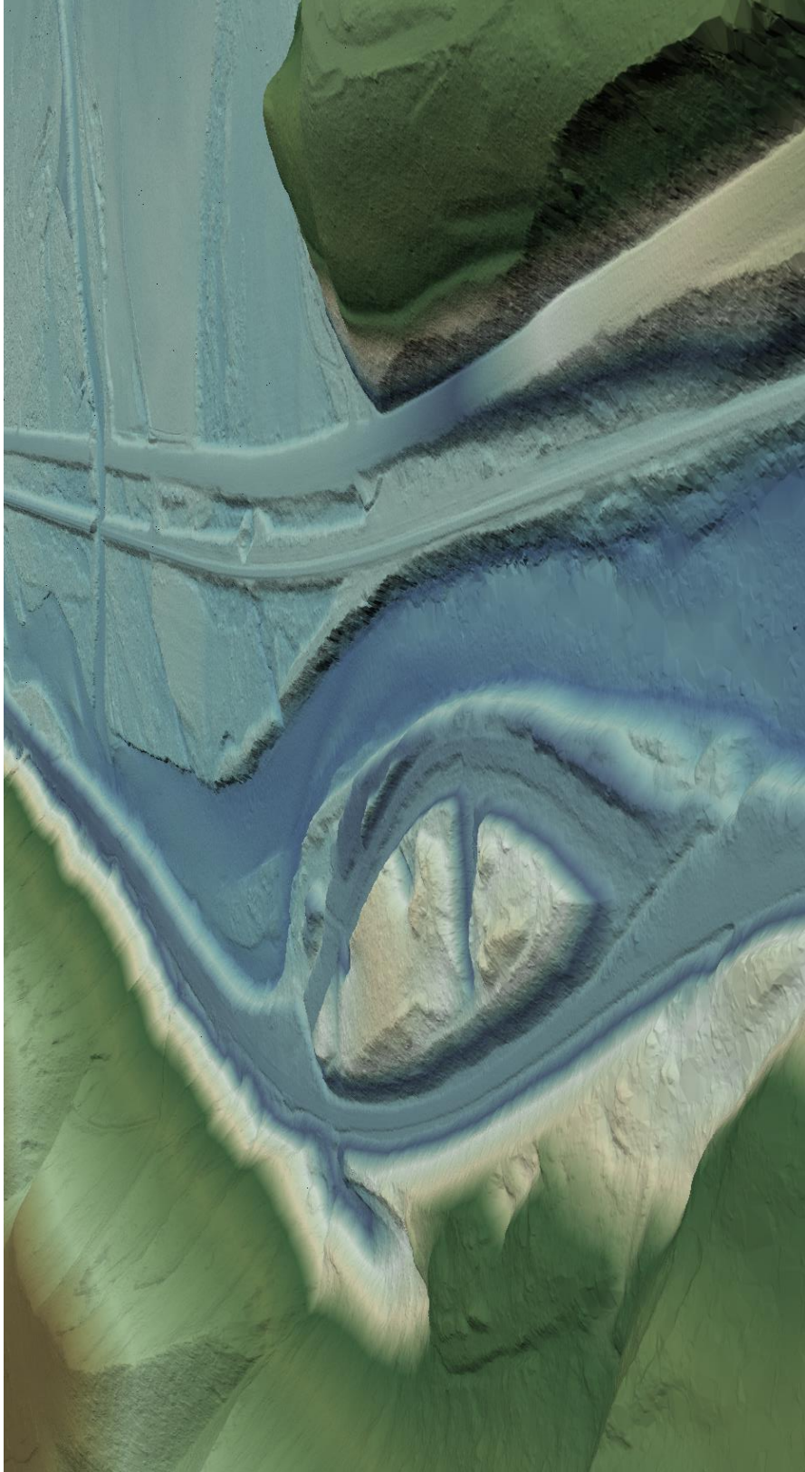
Figure 17: This image was created from the gridded bare earth surface colored by elevation
