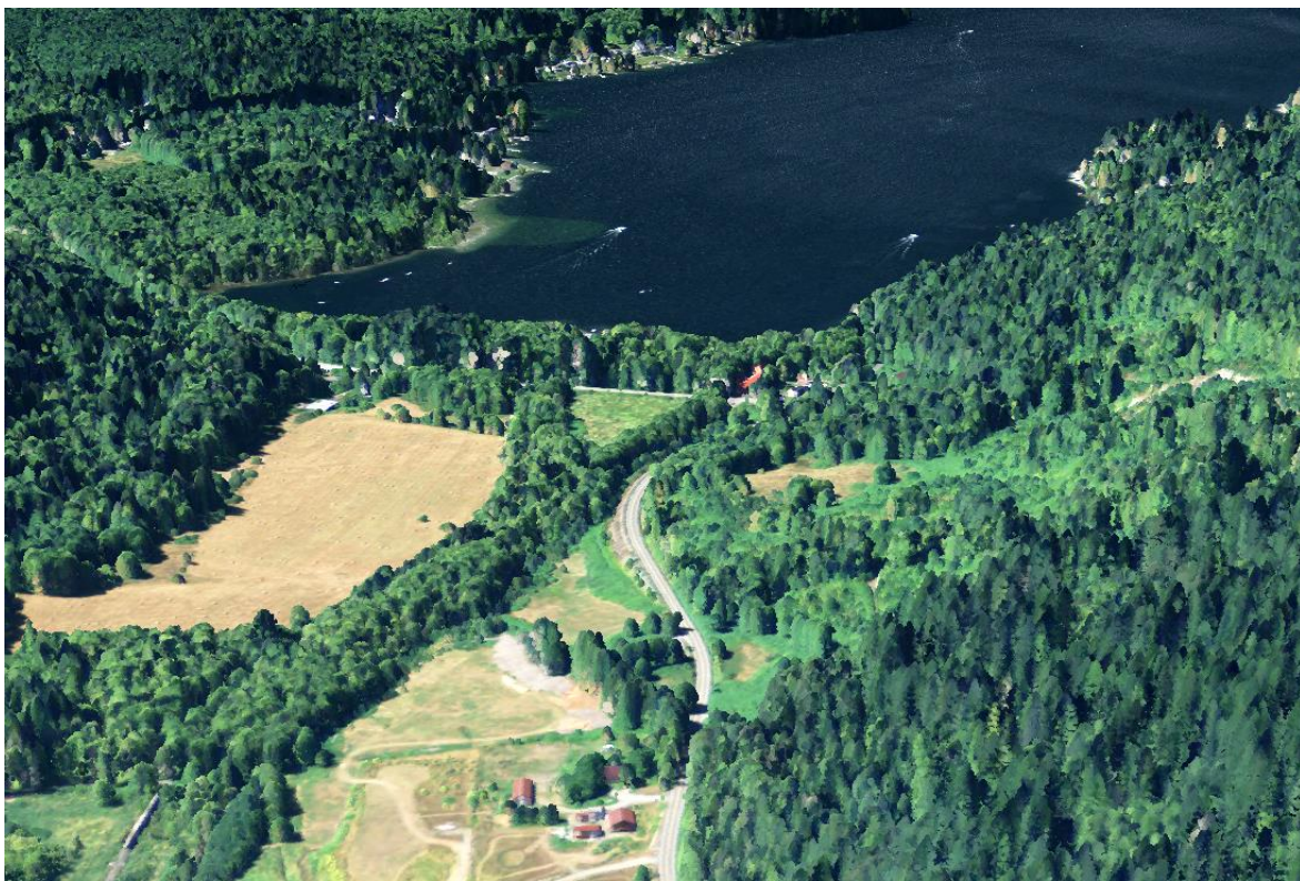
Figure 14: View looking west at eastern shore of Whatcom Lake. Park road can be seen in foreground. Top image created from gridded ground-classified LiDAR points colored by elevation. Bottom image created from LiDAR point cloud with RGB values assigned with 2011 NAIP imagery.
