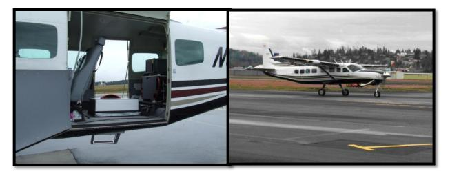
The Cessna Caravan is a stable platform, ideal for flying slow and low for high density projects. The Leica ALS50 Phase II sensor head installed in the Caravan 208B is shown on the left.
