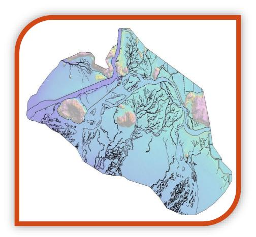
Breaklines for water features are defined in 2D for wider waters and natively in 3D for narrow creek/stream features.
